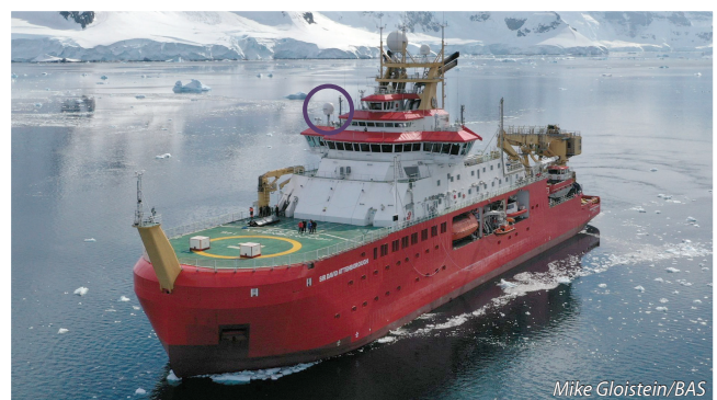
Dartcom Marine X/L-Band EOS System on British Antarctic Survey research ship RRS Sir David Attenborough (antenna circled)
