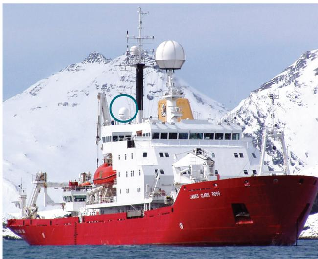
Dartcom HRPT/AHRPT System on the British Antarctic Survey research vessel *RRS James Clark Ross*, with a radome-enclosed active-stabilised marine antenna (circled)
