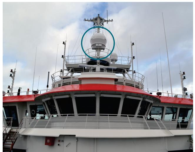
Dartcom 1.5m active-stabilised marine antenna (circled) installed on the oceanographic research vessel BAP Carrasco
